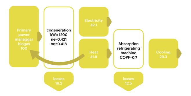
A suggested improvement to the facilities at Balikpapan is the inclusion of trigeneration, a thermodynamic process that creates a simultaneous production of electricity, heat and cooling from a single source. The main difference for Balikpapan is that the cooling produced can be used for air conditioning, a rapidly growing need in Indonesia.
